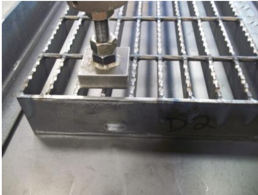
Photo No. 9 Part 2 - IBC Loading -533lb Load at Position 4
