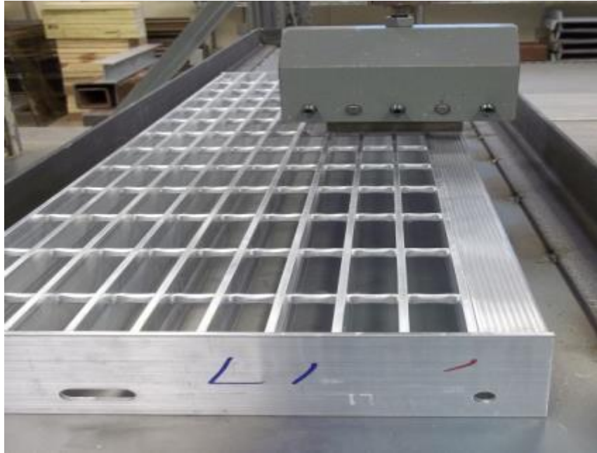
Photo No. 3 MBG 531 Loading - Part One - 300lb Load at Mid-Span
