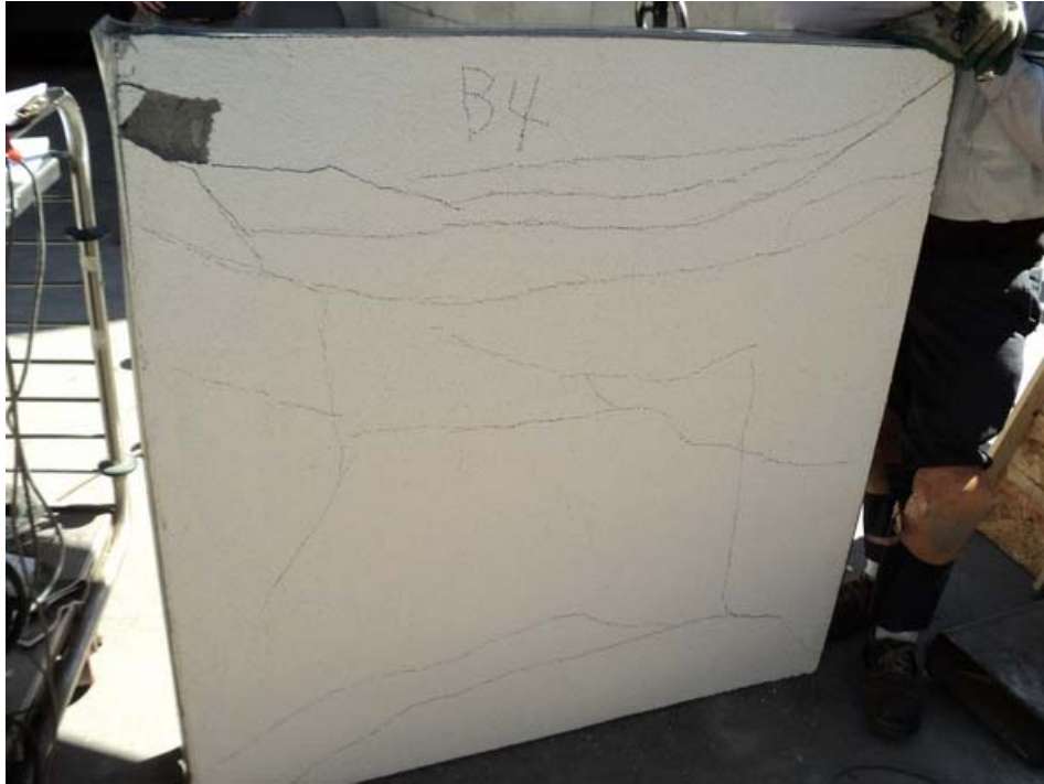
Photo 3 – Typical Failure (B4)
