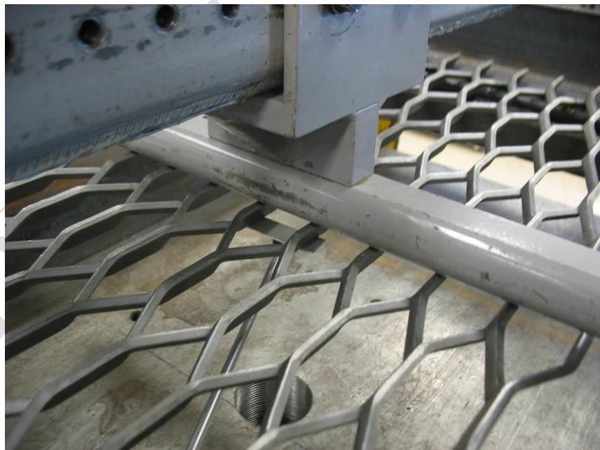
Photo No. 6 Zero Load/Deflection Condition (Post Pre-Load) Loading Rod Contact Detail
