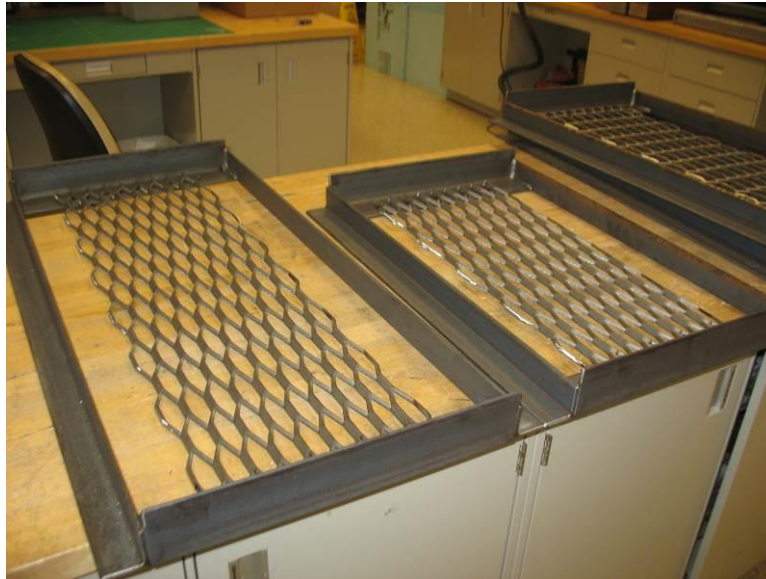
Photo No. 1 Typical Pretest Condition Restriction Frame Reinforced Specimens (3# Product Depicted: 36 in. Span Left, 24 in. Span Right)
