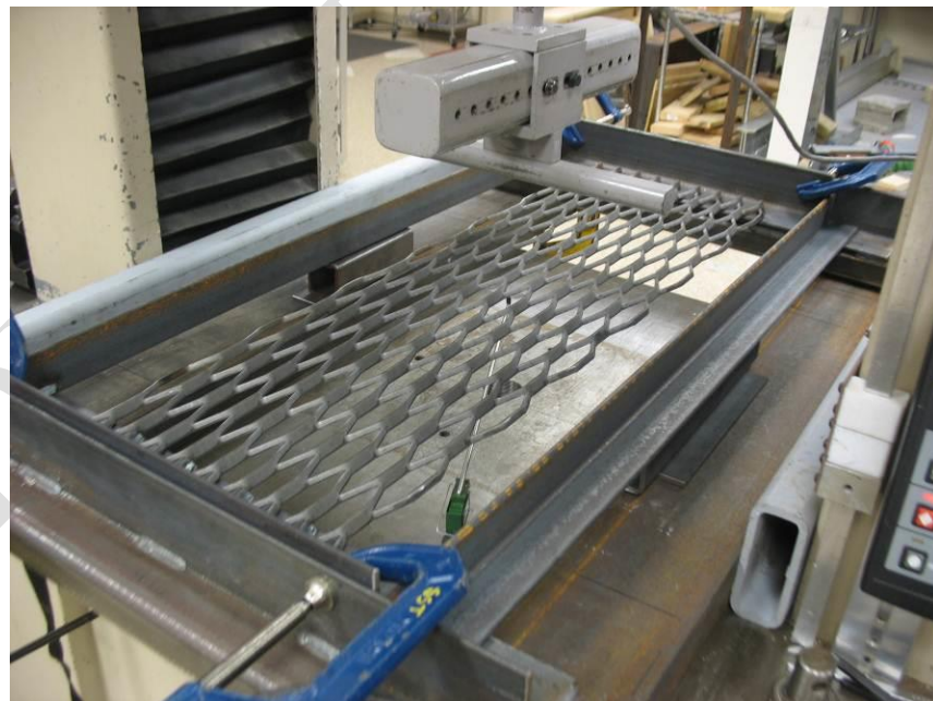
Photo No. 4 Typical 36 in. Span Concentrated Load Restriction Frame Test Fixturing
