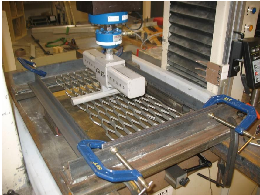
Photo No. 3 Typical 24 in. Span Concentrated Load Restriction Frame Test Fixturing
