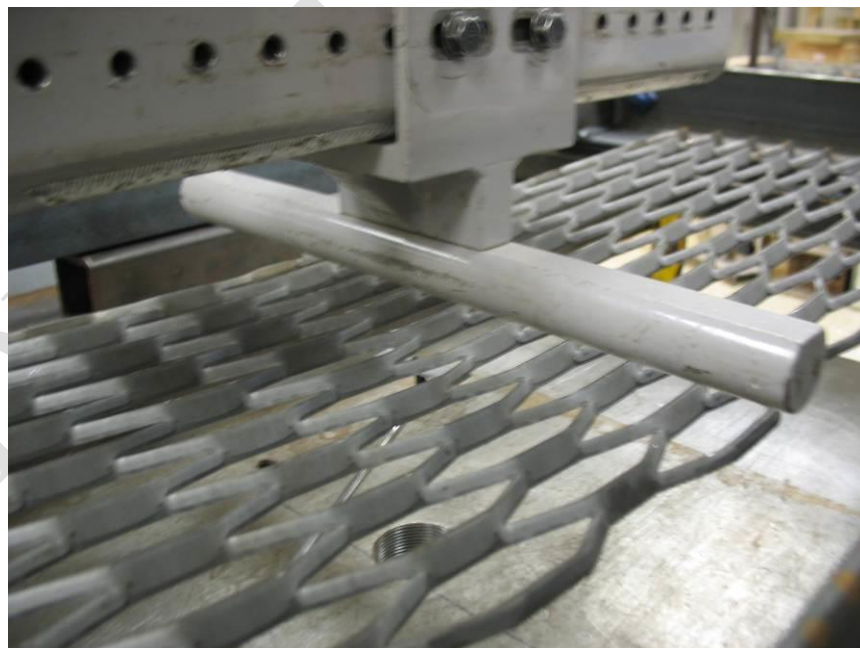
Photo No. 8 Typical Post-Evaluation Specimen Permanent Deformation Specimen Condition (Loading Nose Shown Reset to Pretest Zero Load/Deflection Position)
