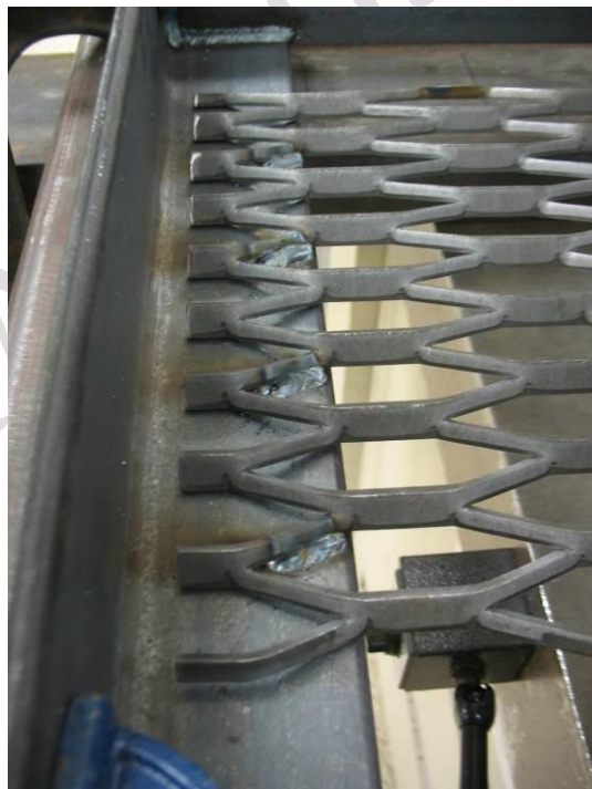
Photo No. 2 Typical Angle Iron Restriction Fixturing End-Weld Detail (Weld-Points to Inside Lip of Angle Iron End-Cap to Define 24 or 26 in. Test Span)
