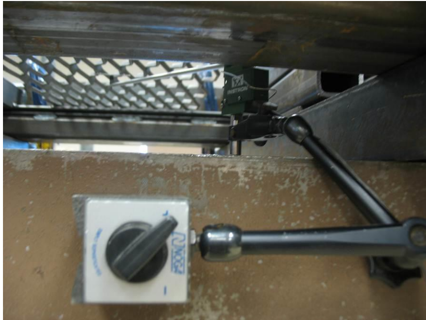
Photo No. 5 Typical Test Setup with Midspan Deflection External Deflectometer in Place
