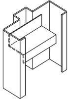
**Z-SHAPED STEEL STUD ANCHORS**
