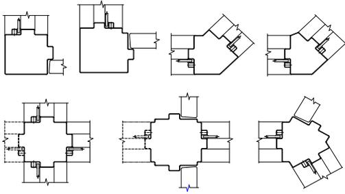
Typical Vertical Hollow Metal Corner Posts for Sidelight and Window Frames
