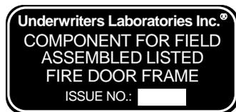
Applied to components of field assembled UL KD, Slip-On or field spliced *frame product*, removable HM *mullions* and panels.
