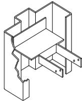
**COMBINATION WOOD OR STEEL STUD ANCHORS**
