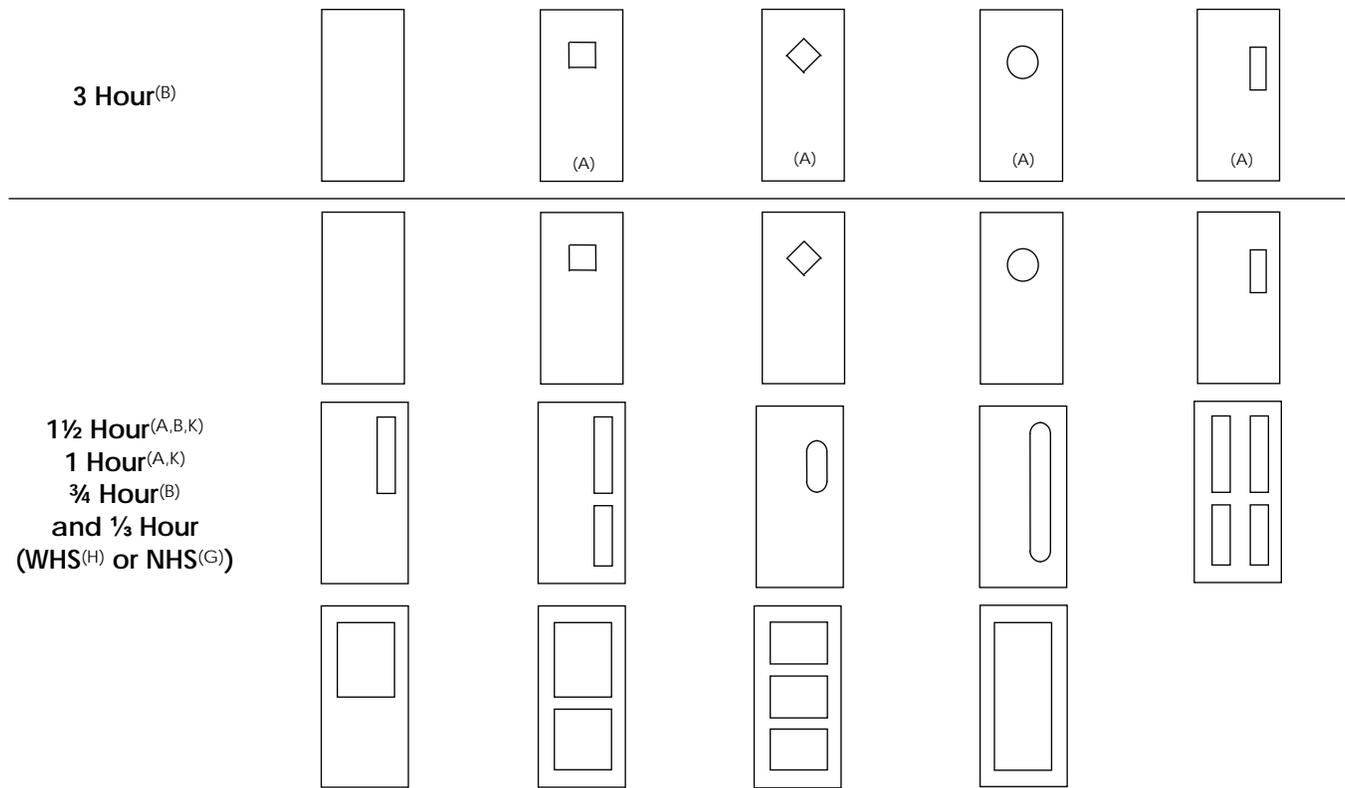
Table 3 summarizes, by *fire-protection or fire-resistance rating*, the maximum areas, widths and heights<sup>(M)</sup> of commercially available *glazing materials labeled by either UL or WH/ITS* for use in positive pressure compliant *hollow metal fire doors*. Users are advised to consult individual *glazing manufacturer's listings* for specific limitations, restrictions, requirements and Human Impact Resistance (HIR) compliance.
